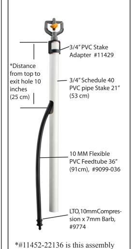
3/4 PVC-5 **PVC Stake Assembly** for 5 mm Tubing Full assembly #11455-12130 includes 3/4" PVC stake - #9305 LTO 5 MM Flexible PVC Feedtube 30" (76cm) #9284-030 3/4" PVC Stake Adapter #11429 3/4" Schedule 40 Distance from top to exit hole PVC pipe Stake 21" 10 inches (25 cm) (not as shown) (53 cm)
