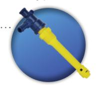
Exclusive Mister Mist'r<sup>®</sup> injection valve with four-way release delivers accurate amounts of concentrate right into the middle of the water supply pipe. Mister Mist'r is also a check valve that helps prevent unwanted leakage or back flow contamination for increased safety. Versatile bleeder/needle valve adds even more convenience, control and safety to the injection process.
