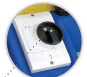
The control switch is sized specifically to each motor and provides overload protection. The switch enclosure is NEMA 4 rated. The control switch is fully integrated into the **Nomad** base.
