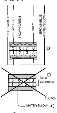
To connect PUMP PRIMING, remove the male connector, insert the connector with the wires brown/blue yellow/blue.
