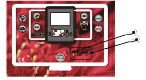
Insert the SIM Card only when the two green LEDs present in the SIM compartment are off.
