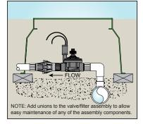
**APPLICATION EXAMPLE:** Placed downstream of the valve and/or filter assembly, the Nelson pressure regulator can provide years of trouble-free pressure control.
