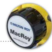
Large, easy-to-read dial lets you adjust flow, quickly and simply, while pump is running. Can be locked in position to maintain constant flow. Precision stroke adjustment can be operated while in use. Steady State Accuracy ~ + 2% of full capacity over the 10 to 1 turndown ratio.
