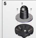
Install new plate by aligning all three holes in the backer plate with the holes in the plate and inserting three screws.
