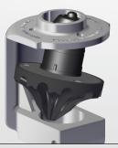
7 Secure plate/motor assembly to body by replacing the snap ring.
