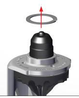
Separate plate/motor assembly from body.
