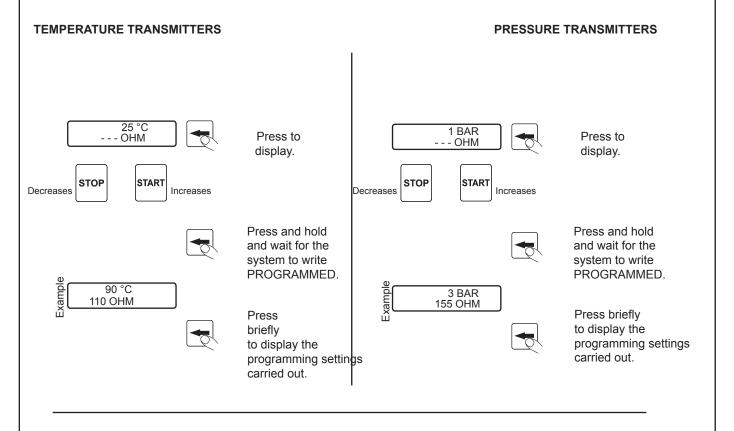
WARNING: It is necessary to program at least 2 values (to obtain good precision in the control of temperature and pressure, we recommend programming at least 4 values).
