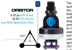
The Orbitor features new technology that eliminates the struts of a sprinkler body to provide outstanding uniformity and optimal droplets at low operating pressures. Designed with an innovative, bracketless assembly, debris hang up and water pattern misting common to conventional sprinklers are mitigated. 3000 Series (3TN nozzle) or 3030 Series (3NN nozzle).
