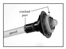
6. The plunger is tested for damage by inserting the end of a pencil inside the inlet end. Check the retainer for cracks also.
