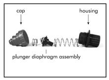
**4.** The major parts are the cap, housing, plunger/diaphragm assembly and springs.
