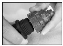
**8.** Reassemble being sure to tightly screw together the cap and housing which seals the regulator.
