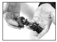
**5.** Leakage of water between the cap and housing is an indication of a split plunger.
