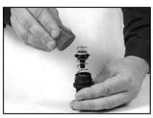
**7.** A broken plunger/diaphragm assembly can easily be replaced with a new plunger/diaphragm assembly.
