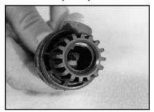
**1.** Check inlet and seat area for debris plugging. Remove any debris.
