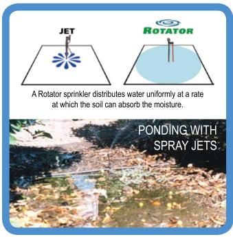
Rotator systems can be designed to easily meet E.T. requirements and still deliver water to the soil gently in the range of .04 to .15 in/hr (1 to 3.8 mm/hr). A uniform light application rate Rotator full coverage system can be combined with applications of gypsum and other soil amendments to vastly improve soil infiltration problems.
